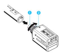
Tighten the locking ring 2 as shown.
